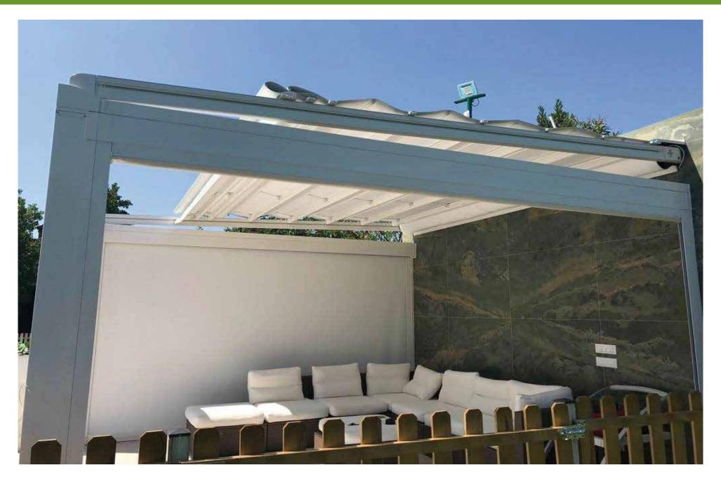
It is a pergola with a modern and linear design, versatile and easy to install, with high quality standards. Entirely made with painted aluminum profiles and with pre-tensioned blackout PVC covers, or embossed Valmex blackout PVC or two-colored Opatex PVC, the structure is wall-mounted and moved by a radio-controlled electronic motor, which allows the upper folding opening of the single fabric up to maximum tension.
